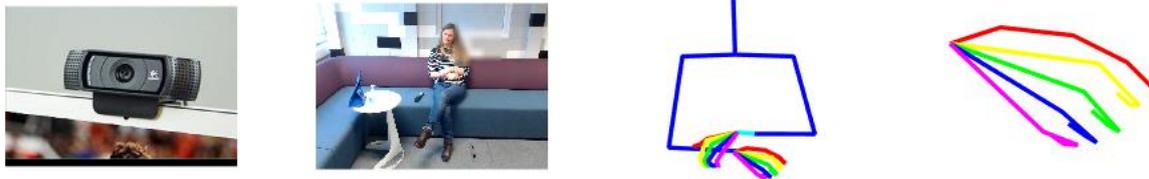
**Figure 8:** With a camera placed above the TV screen, the subject is recorded whilst seated, watching TV. OpenPose is used to estimate hand and body keypoints.
