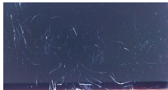
Figure 2: phone screen scratch images taken using a digital microscope
