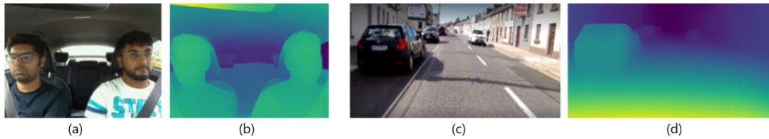
Figure 4: Depth Camera Sensor Outputs. a) In-cabin RGB camera b) Corresponding in-cabin depth output c) Out-cabin RGB camera d) Corresponding out-cabin depth output.
