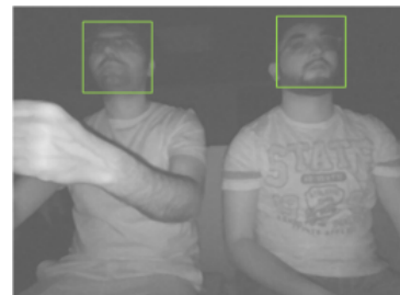
Figure 2: NIR output for monitoring the driver and passenger
