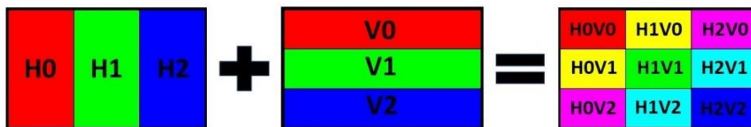
Figure 3: A diagram illustrating how the combination of a 3x1 and a 1x 3 model is equivalent to a single 3x3 model.
