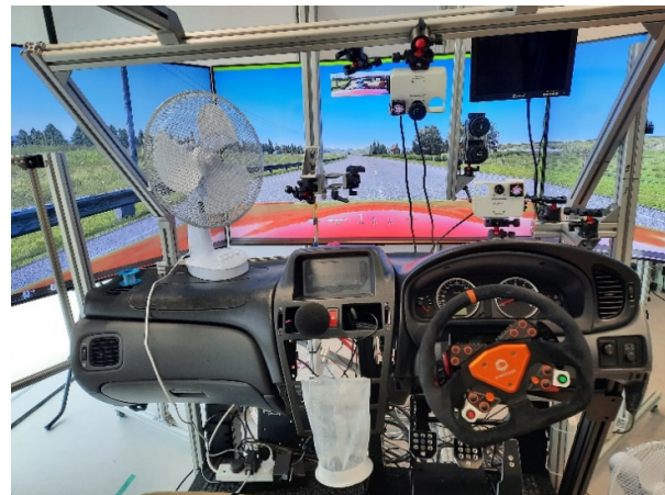
Figure 1(b): Driver view with instrument cluster, steering wheel, pedal assembly and video acquisition systems
