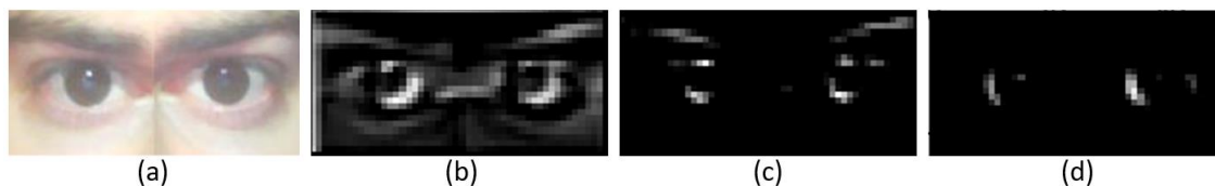
Figure 2: Example of the input image and feature maps produced by 3 different models. (a) input image, (b) activation map generated by a single 3x3 model. (c) activation map generated by 1x3 model focused on determining vertical position. (d) activation map generated by 3x1 model focused on determining horizontal position. White pixels represent pixels of significance. Note for (c) and (d) the areas of significance around the sclera of the pupil, and the lack of weighting on other, irrelevant features.
